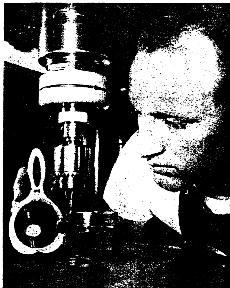
Reflecting the skill and care that goes into the intricate tools, dies and fixtures turned out by the skilled craftsmen at Sheaffer's Tool & Die plant is this shot of Dale Yantis checking a job on a SIP jig borer. Today, in addition to meeting the company's needs for precision dies and tools for the manufacture of writing instruments, Sheaffer's Tool & Die Division produces tools, dies and fixtures for many major companies throughout the nation.
